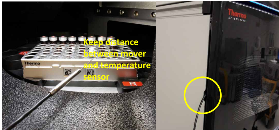
Figure 25: Positioning the temperature sensor in the vial (here: Vanquish autosampler); the sensor cable can be led out at the left door side
