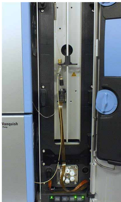
Figure 29: Installed Active Preheater TQ OQ Kit connected with preheater to be qualified, waste capillary is directed to the system drainage system.
