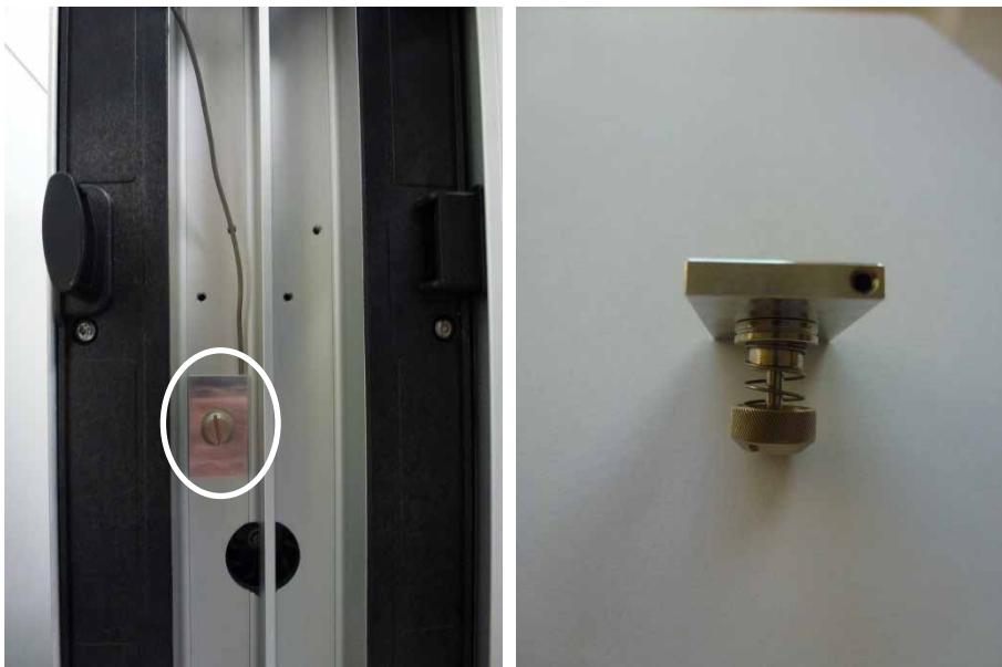
Figure 11: Left: VC-C10-A and VH-C10-A-02 (revision 02) – Position of the temperature sensor; Right: temperature sensor mounting bracket that has to be mounted manually in the compartment for qualification purposes
